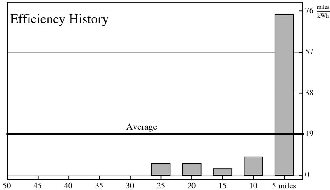
Figure 3. Actual rendition of a screen that the Bolt presents the driver in the hope of communicating the average consumption over 25 miles. The value of 19 is grossly incorrect. The correct value is 6 mi/kWh.
