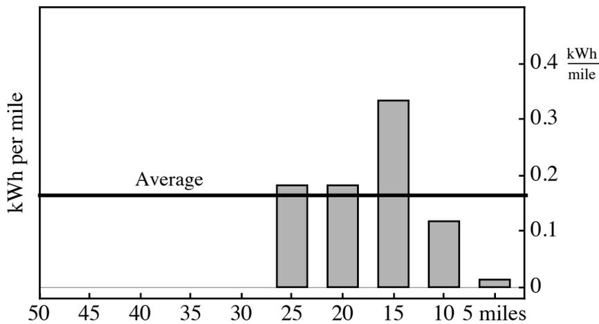
Figure 4. In the inverted system (kWh per mile) the bar heights give an immediate visual feel for the average energy consumption.
