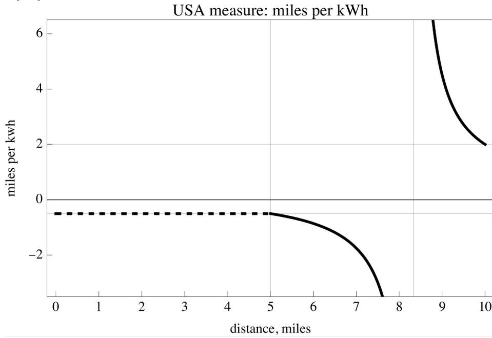
Figure 1. The fuel consumption for a drive of 5 miles downhill followed by 5 miles gentle climb, measured in miles per kWh.
